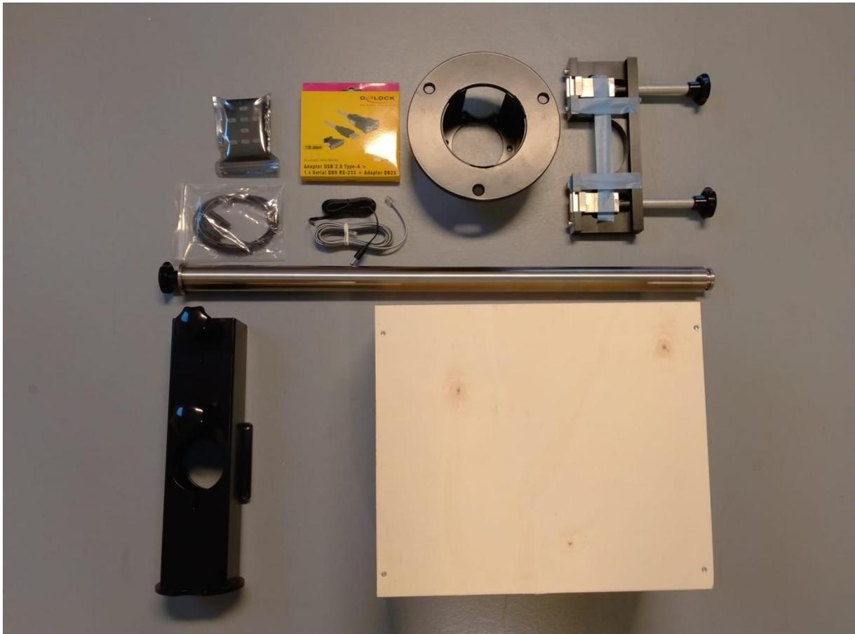
*The basic parts to set up your Mesu mount. (from top left to Bottom right, reading order): SiTech handpad, serial to USB adapter, Base plate, Saddle plate, Connection and power cables for Sitech controller, Counterweight bar, Counterweight box, Crate containing RA and DEC drive units.*
