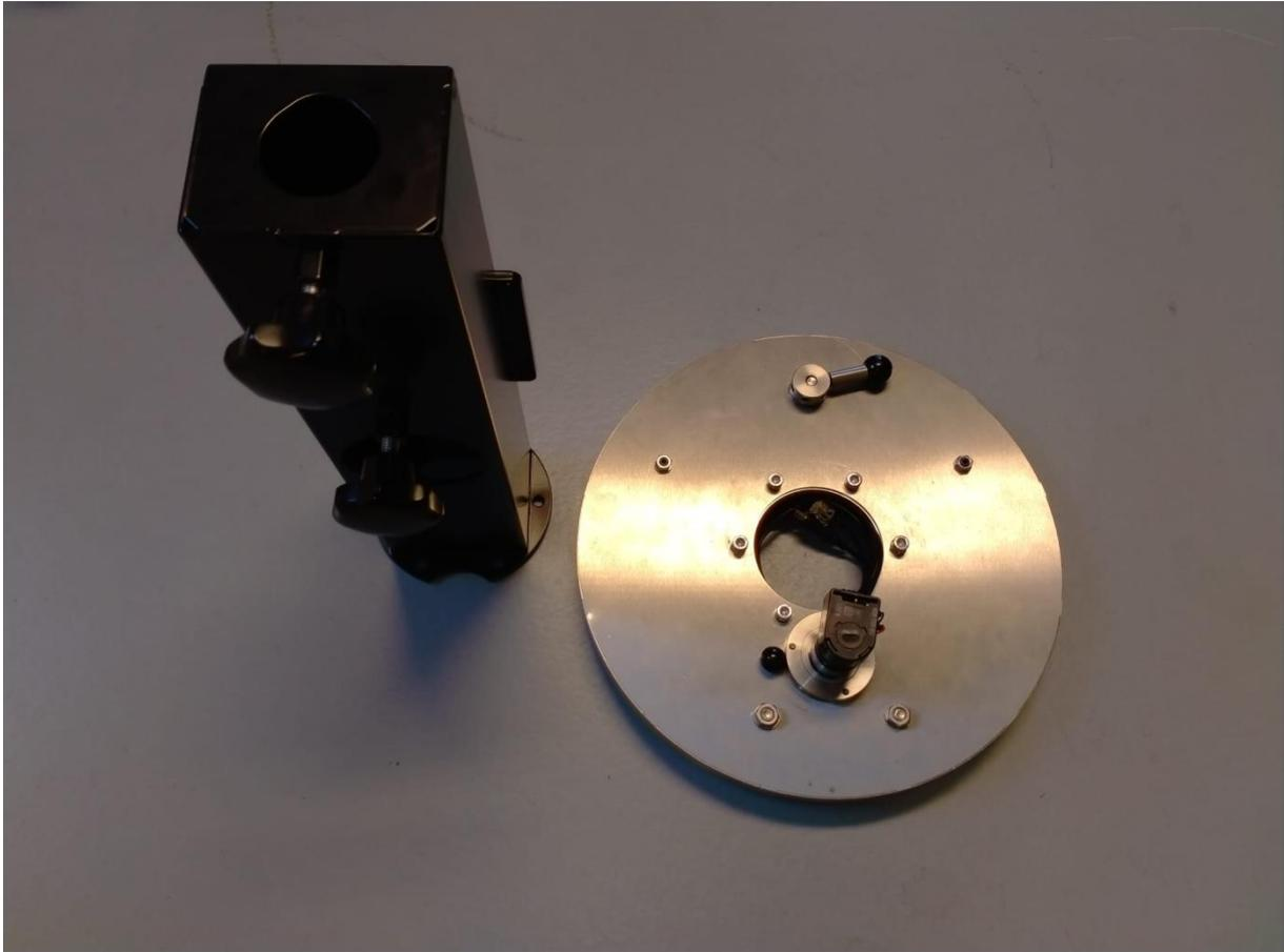
Six Allen bolts have been put in the centre of the DEC unit, two of which have an extra nut and are tightened. Unscrew the six centre bolts and remove the two extra nuts. **These two nuts were only for transportation, and are not necessary for constructing the mount.** Place the counterweight box on the DEC unit and screw the six Allen bolts back. Make sure no cables are wedged in between the DEC unit and the counterweight bar box.
