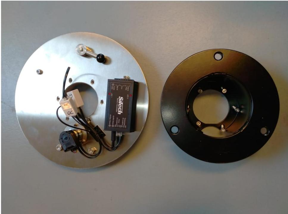
As with the DEC unit, six Allen bolts of which two have nuts are screwed in the centre. Unscrew these, dispose of the two bolts, place the base plate on the DEC unit and screw the Allen bolts back in. When doing this, make sure the protruding cables are not wedged in between the unit and the base plate, but are sticking through the specially designed hole:
