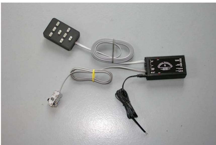
The 12V cable needs to be connected with the dotted line to the + and the other to the – 12V DC. Voltage needs to be within 12 and 18 V DC. 2 Amp is more than enough for moving both motors at the same time with the highest speed. A good size battery would for example be the battery of a motorcycle.
