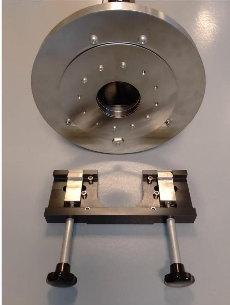
Remove the tape and bolts, and mount the saddle plate to the RA unit using the six remaining holes.
