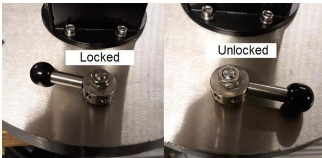
The brakes at the other side of the housings can be unlocked by turning them counter clockwise. When you rotate the Dec. brake as far as possible it can't walk back when using the mount. In that position the two axels can be rotated for balancing your setup. You can start by locking the dec and balance the RA or in another way you prefer.
