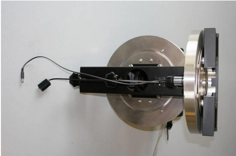
Find the rectangular connector plug which has DEC written on it, and connect the DEC encoder cable. Following the other wires to the Sitech controller, connect the DEC motor cable to the remaining Sitech controller port.
